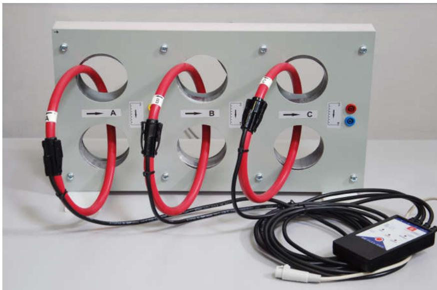
**Note! The current going through the Calibrated Coils from the CA-3.1 amplifier shall not exceed 10A.**
