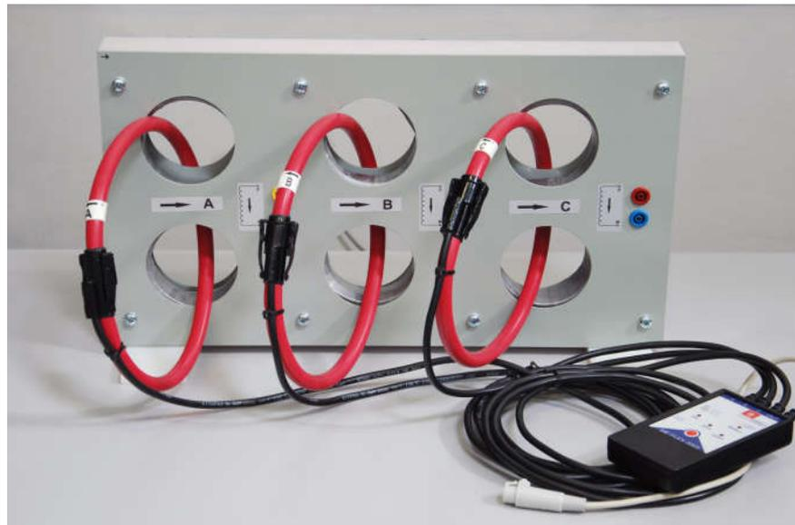
Fig. 2.16 100-Turn Calibrated Coils
